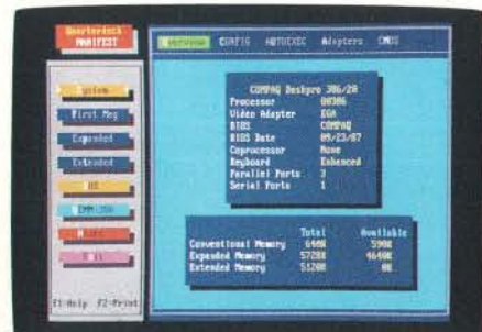
Manifest shows you how your memory works. Here's the first megabyte of RAM, showing unused areas.
